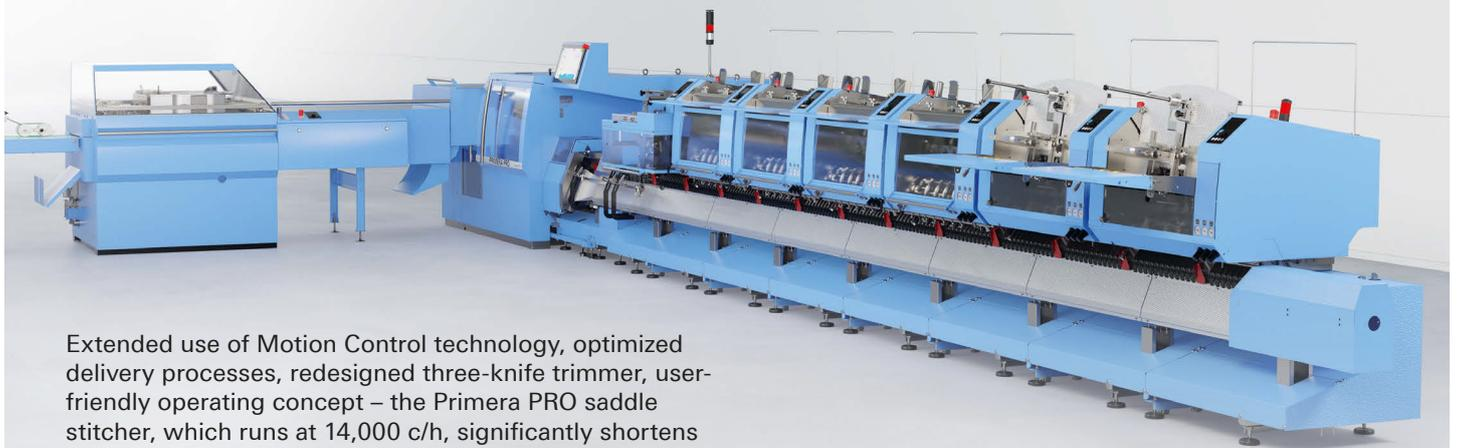
Extended use of Motion Control technology, optimized delivery processes, redesigned three-knife trimmer, user-friendly operating concept – the Primera PRO saddle stitcher, which runs at 14,000 c/h, significantly shortens the set-up and throughput times of your jobs and thus increases your profitability. Thanks to its high format variability and the large selection of feeders, it is the ideal saddle stitcher for a wide range of products - for short runs as well as longer runs.
