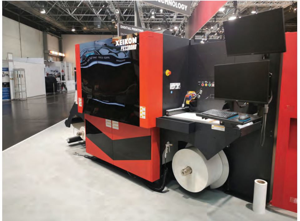
Zeikon Panther PX3300HD—UV inkjet label press Zeikon Panther PX3300HD-UV-Inkjet-Etikettendruckmaschine
