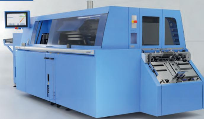
The Vareo PRO perfect binder is the most ideal perfect binder for print finishing specialists and printing plants that use conventional printing modes or are engaged in digital printing. Whether for medium, short or ultra-short runs, right down to runs of one copy, the Vareo is an all-rounder and stands for outstanding binding quality. The first book produced with the three-clamp perfect binder is already available for sale.
