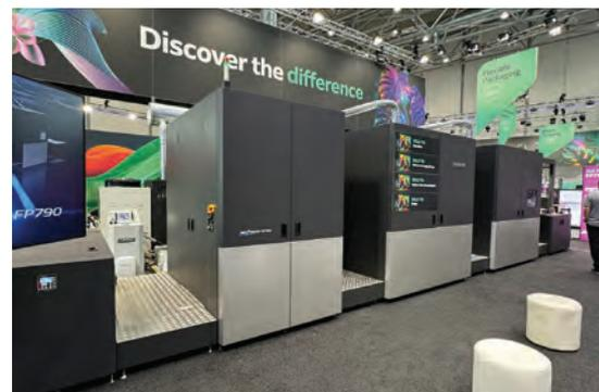
In the wide-format space, the new Acuity Triton and the Ultra Hybrid with automation, now use AQUAFUZE ink technology which combines the benefits of UV LED and water-based inkjet. It has low-energy, low-temperature drying compared to traditional water-based print systems and provides excellent adhesion to a wide range of media without the need for a pre-coat primer or optimizer.
