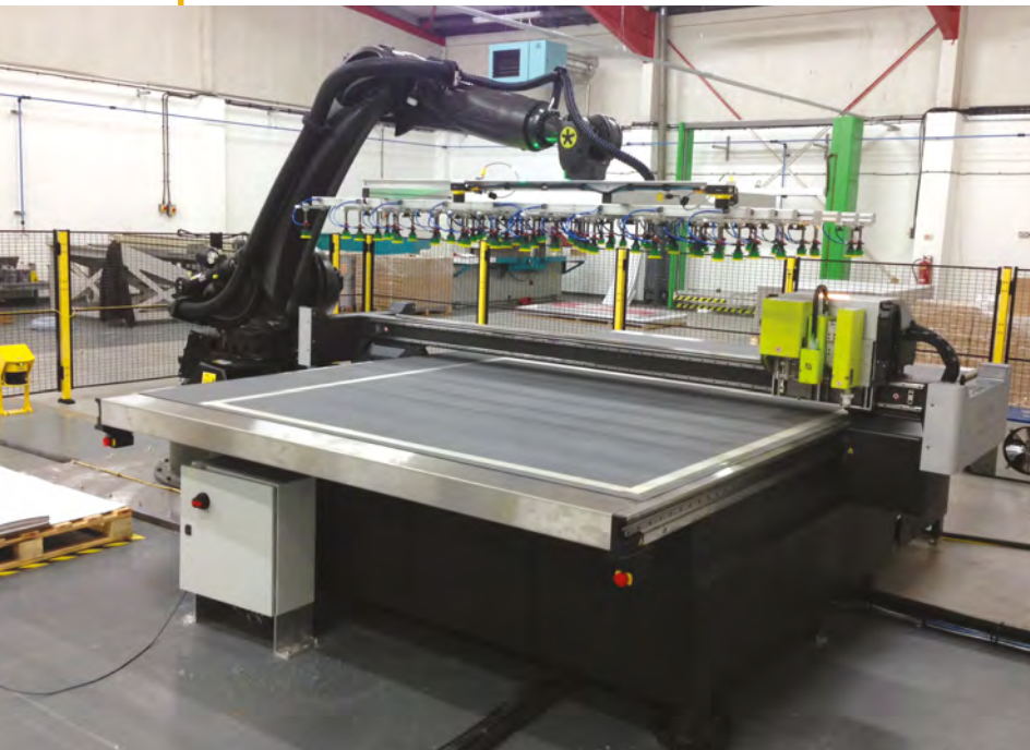
The Kongsberg cutting table (formerly developed by Esko before Kongsberg was spun out as a separate company) added a robotic arm for loading and unloading several years ago.
