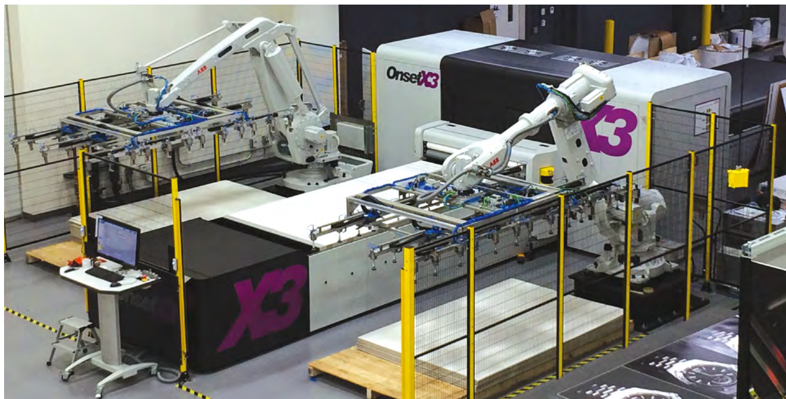
Two arms good: Inca Onset with dual automation system. (Image courtesy Fujifilm)
