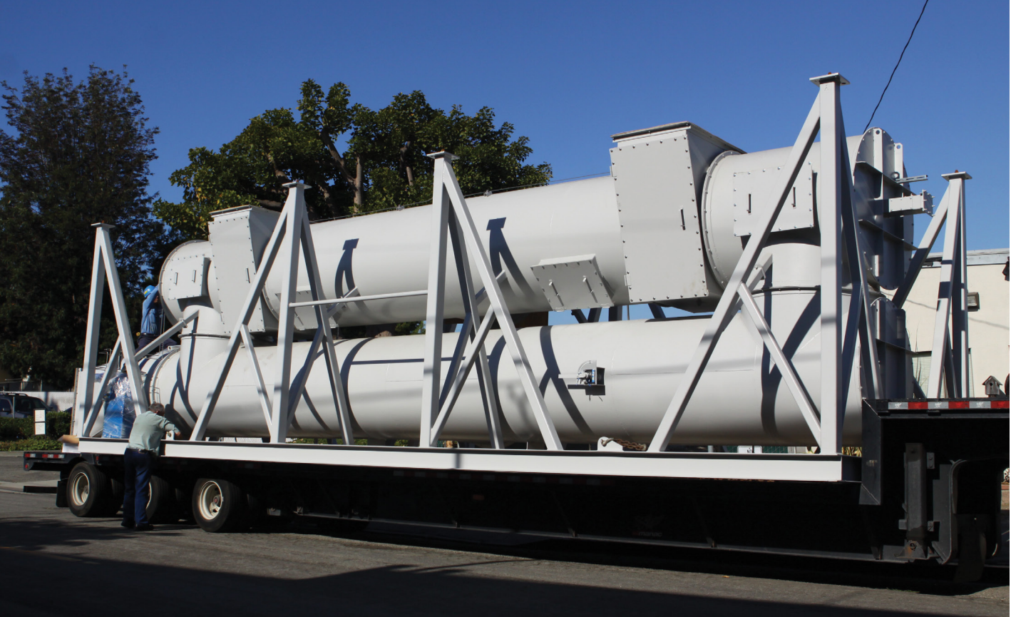
Modular Construction of an RTO Inlet and Outlet Manifold for fast and easy bolt together construction.
