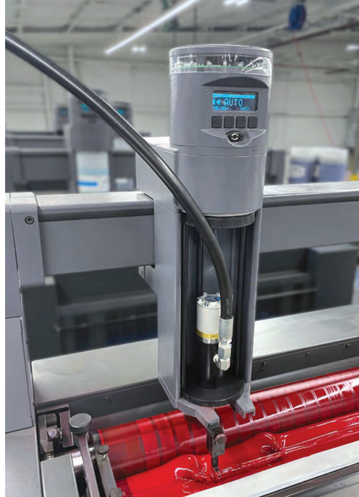
(Above) Swapping out an ink canister takes only 10 seconds. (Right) The Sentinel RemoteLinc adapter draws ink directly from bulk supply drums.
