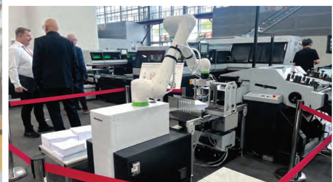
Horizon's robot arm system for book production.
