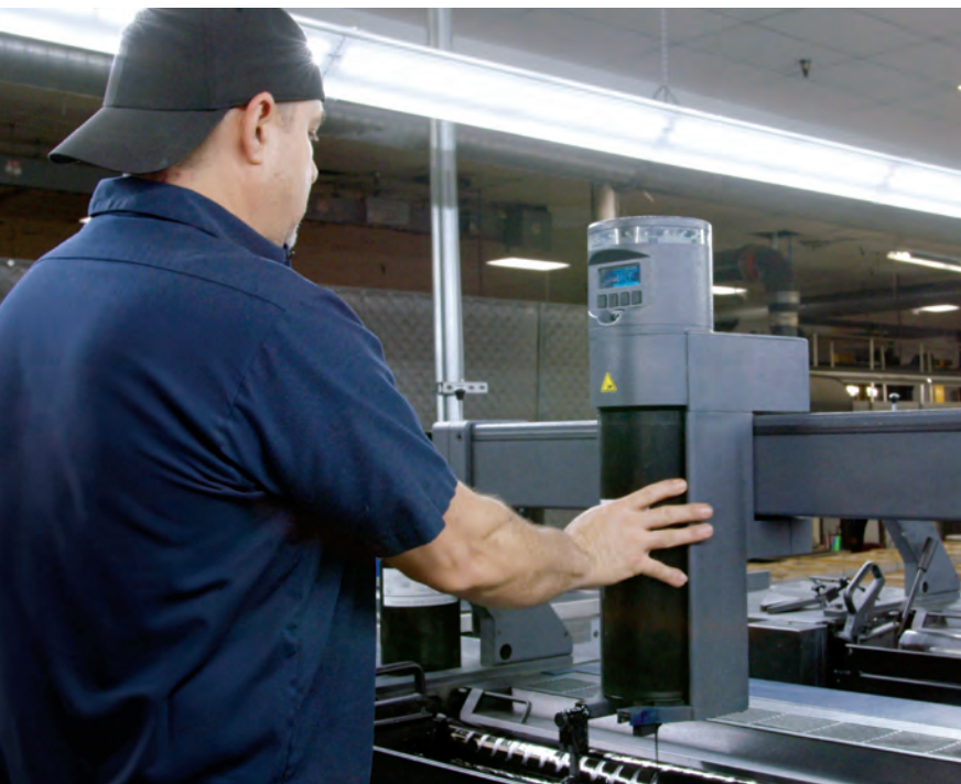
(Above) Swapping out an ink canister takes only 10 seconds. (Right) The Sentinel RemoteLinc adapter draws ink directly from bulk supply drums.
