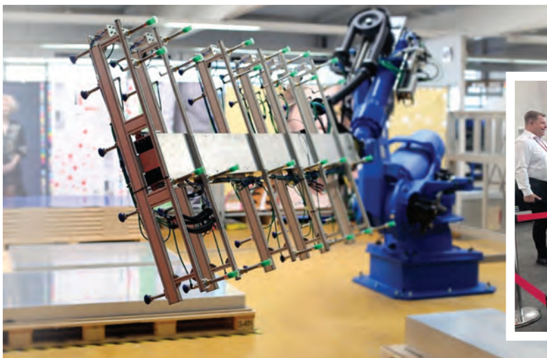
ECO3's plate-loading robot for its Avalon VLF platesetters.
