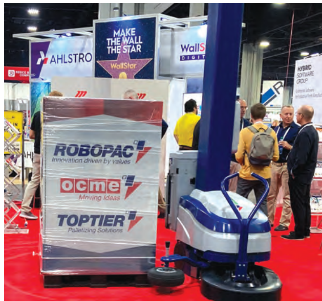
Robopac’s self-propelled stretch-wrapping robot.
