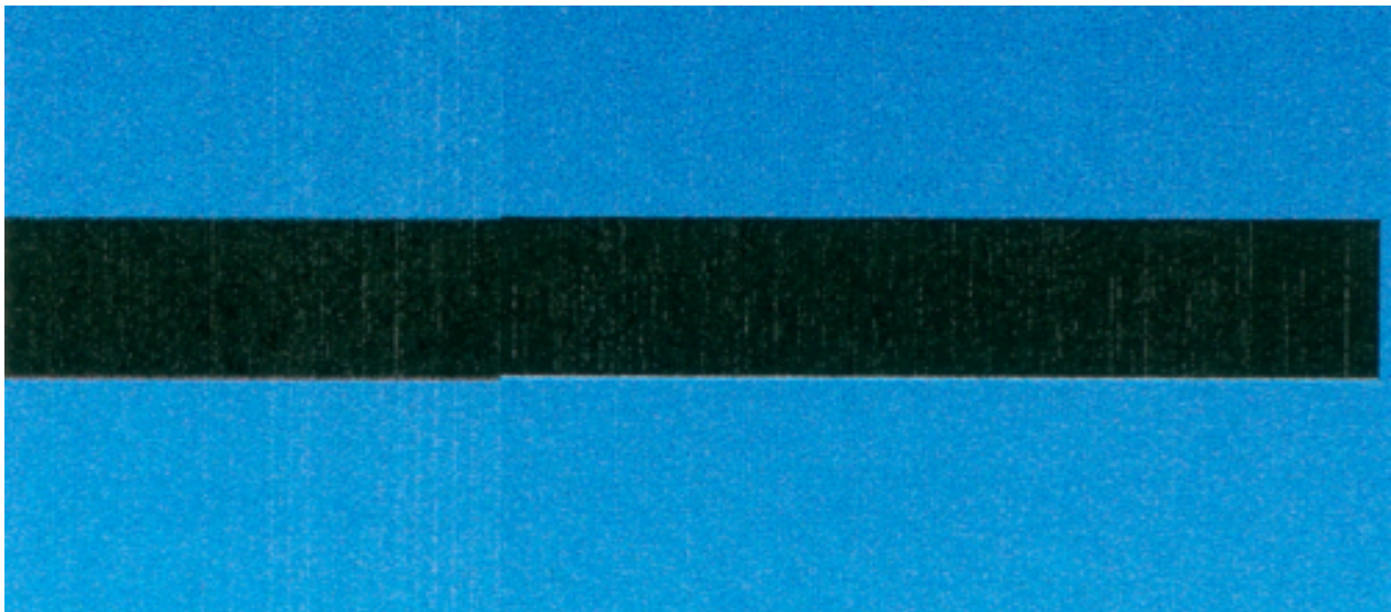
Figure 6: Example of Banding Defect. Sample shows right to left, cross process directional banding
