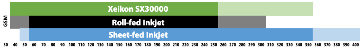
Figure 1: GSM Distribution. Solid colors represent gsm handling at full speed and lighter colors represent reduced speed for toner and/or coverage for inkjet
